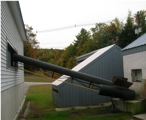
**The old lumber conveyor converted to sludge conveyor**
