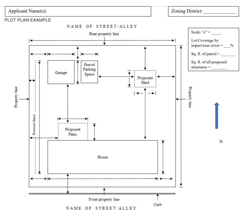
This is an example of a plot plan, in which all structures are existing except for the patio, shed and fence. Please create a plan for the property in which you are applying for a zoning permit by showing the property line boundaries along with all existing and proposed structures. Your drawing must be to scale, and must be an accurate portrayal of an overhead view of the property. Please submit one copy of your drawing with the permit. Your scaled plot plan/survey must include:
